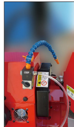
Separate Cooling System
