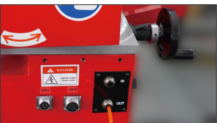
Air Pipe Port & Electric Port
