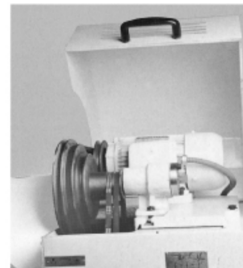
Head stock speed quickly change belt
